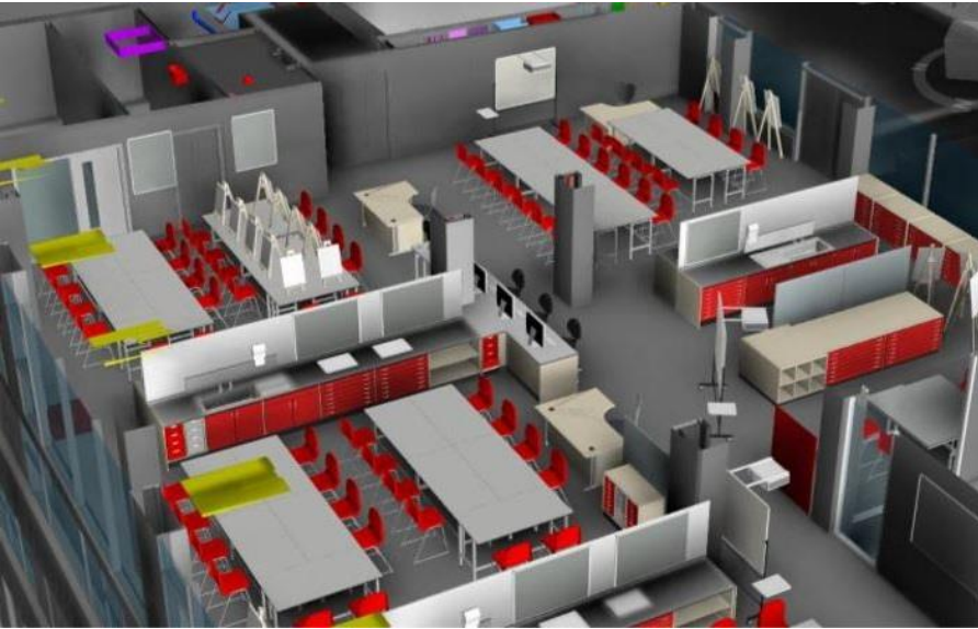
Images (L) The FF&E3D model was utilised for stakeholder consultation, RDD sign off, and coordination with the design models. (above) Coordinated MEP systems and framing were modelled digitally and fabricated off site. Model data was used to check tolerances and simulate virtual installation sequences.
