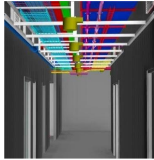
Images (L) The FF&E3D model was utilised for stakeholder consultation, RDD sign off, and coordination with the design models. (above) Coordinated MEP systems and framing were modelled digitally and fabricated off site. Model data was used to check tolerances and simulate virtual installation sequences.
